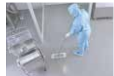
Sealed special fibres prevent the emission of particles.
