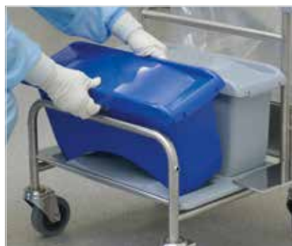
8 Activate the next system box with prepared mops, etc.
