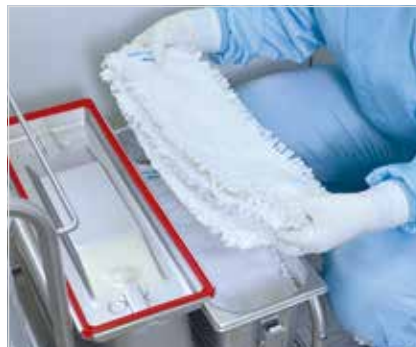
2 Load the system box with no more than 10 mops – ensure that the back of the mop (pocket) is pointed up
